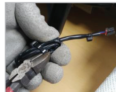
④ Cut Cable tie
